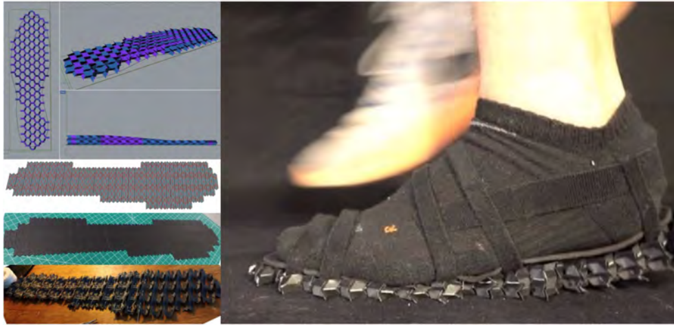
Figure 2: A) Digitally designed geometry for shoe sole, B) Cut pattern for shoe sole, C) Laser cut polypropylene prototype, D) After initial folding, E) Testing the shoe sole at running speed.
